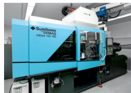
Fig. 7. The test machine is an all-electric injection molding machine with integrated simultaneous compression control
