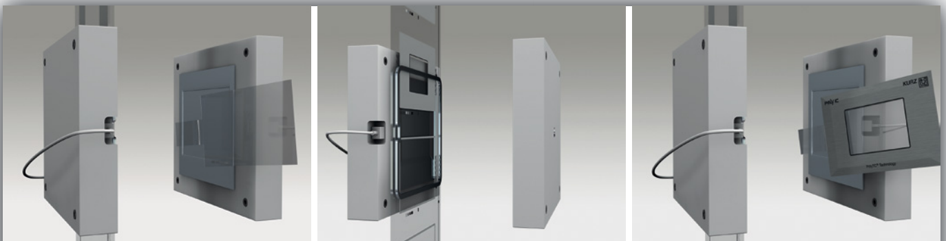
From left to right: Placing of the PolyTC IML label on the injection side of the tool; Positioning of the decorative foil; Removal of the finished touch sensitive display
