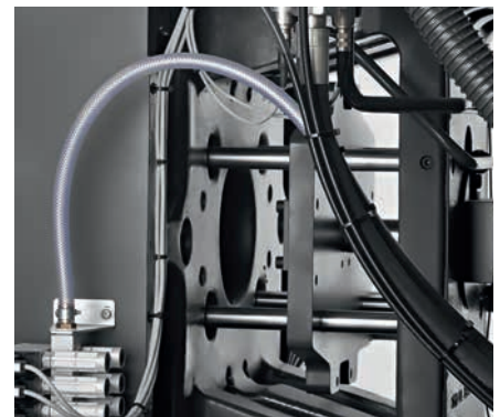
High-speed ejector with position control
