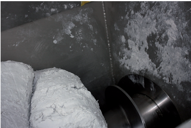
In the tamper, the BMC material, which has the consistency of sauerkraut, is introduced into the plasticising unit with a stuffer screw and then fed to the actual feed and injection screw.
