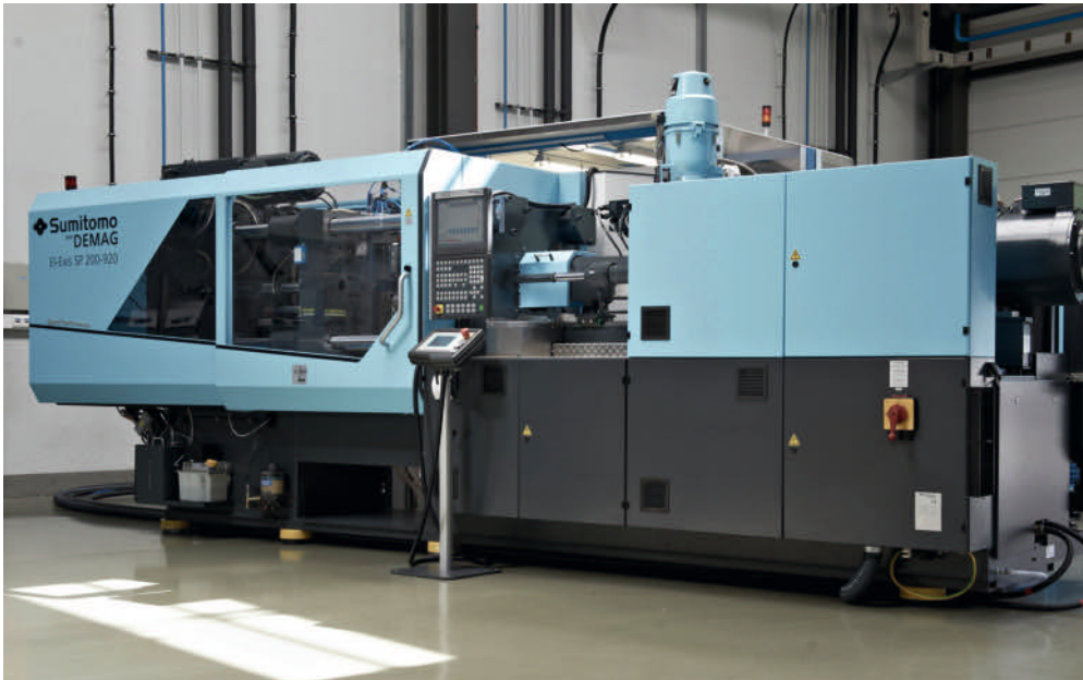
Fig. 1. The hybrid-drive high-speed EL-Exis SP injection molding machine – in this case with 2,000 kN clamping force – has further improved dynamics compared to the preceding series (photos: Sumitomo (SHI) Demag)
