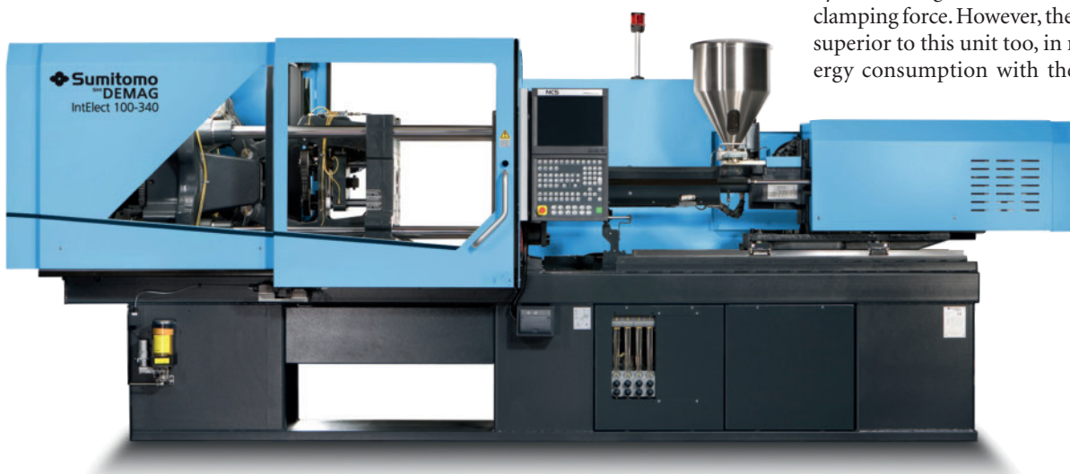
Fig. 2. Making use of an all-electric injection molding machine gives production benefits due to the high degree of operation precision, in addition to significant energy saving. The photo shows an IntElect 100-340 machine (figs.: Sumitomo (SHI) Demag)
