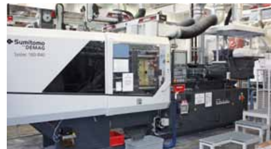
The poly-stuffer for loading the material (right) as well as the large extraction systems above the stuffer and mould area are the most striking differentiating features compared to the thermoplastic injection moulding machine.
