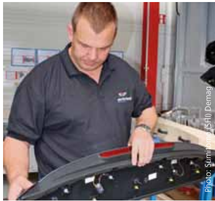
Karl Menrad inspecting a rear spoiler. Autotest Eisenach combines injection moulding technology and polyurethane processing for such components.
