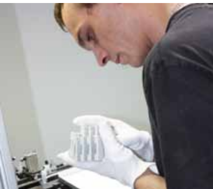
A production employee takes samples of the parts for visual inspection before they are transported to the flash removal system.
