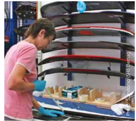
After the bumper parts have been painted at an external partner, they are quality-checked at Autotest and then glued together.
