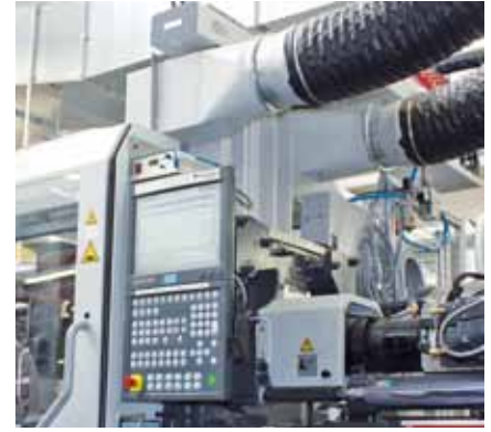
The extraction system removes not only the reaction products but also other gases which would interfere with filling.
