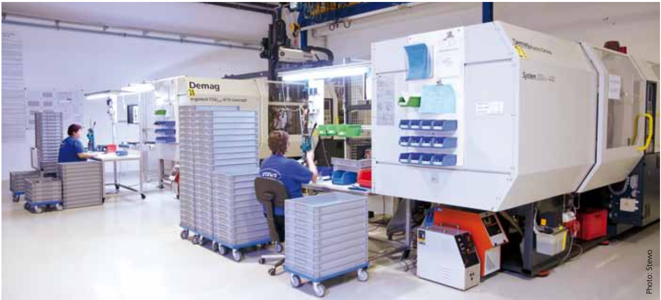
A linear robot removes the lever and places it on a conveyor belt. After a defined cooling line, the employees fit a pin and a greased spring on the levers; they perform a visual check and place the parts in the grey trays.
