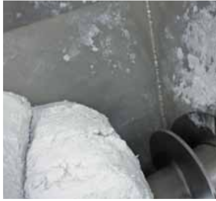
In the poly-stuffer, the BMC compounds with the consistency of pickled cabbage are transported into the plasticising unit.
