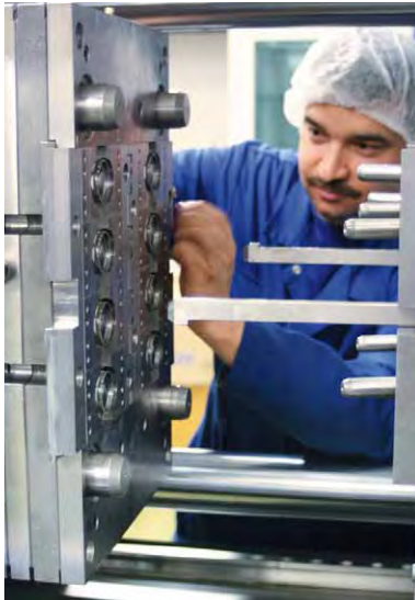
Multi-cavity moulds: An eight-cavity hot-channel mould during setup
