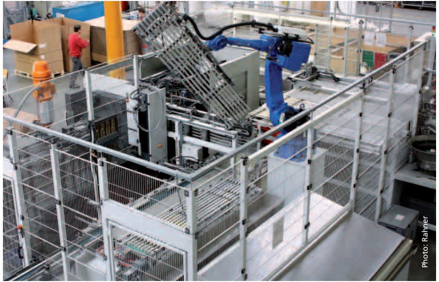
The corrugated tubes which have been cut off are transported into the automation area via a conveyor belt (left below) and are fed into the injection mould in batches of eight units each via an articulated robot.
