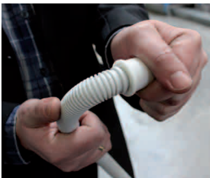
Through the injecting of sole of the flexible pipe collar made of TPE onto the PP tube, both a positive and also a firmly bonded connection is created, which ensures total water-tightness when the dishwasher hose is attached to the siphon.
