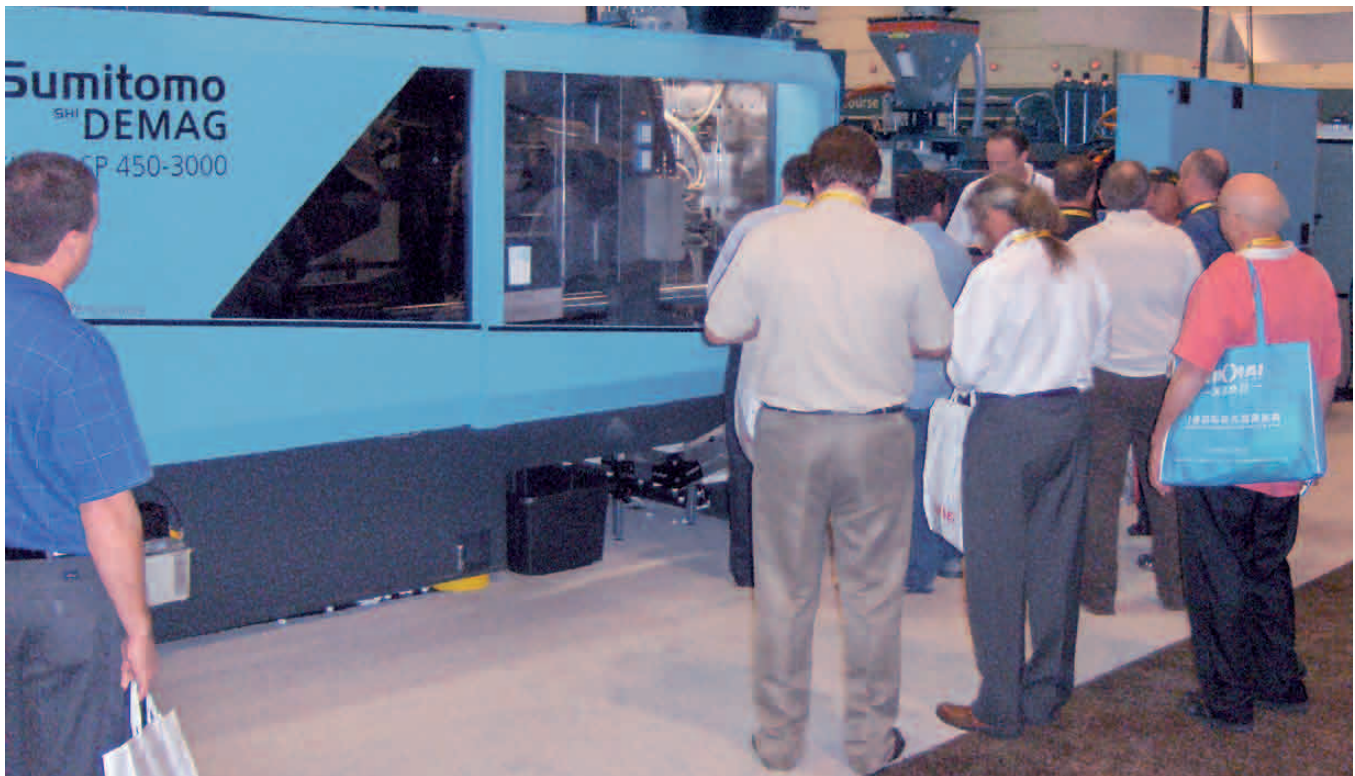
Impressive exhibit: At NPE in Orlando, an EI-Exis SP with a clamping force of 4,500 kN and a 96-cavity injection mould of Schöttli AG produced screw caps in a cycle time of only 1.95 seconds.
