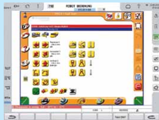
Virtual Network Computing (VNC) will integrate robots made by Wemo into the NC5 control
