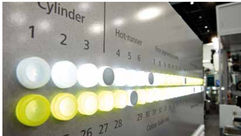
A production study demonstrated fast colour change in the use of liquid dyes instead of master batch
