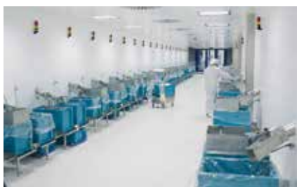
Cleanroom in the lower basement for packaging of the products, which arrive there via transport pipes
