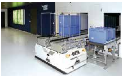
Driverless transport system for the collection of containers at an intermediate air lock
