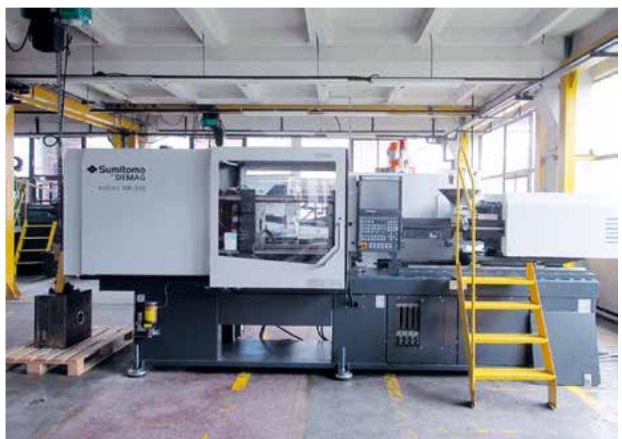
Plastor was convinced by the high precision, high speed and low noise level of the fully-electric injection moulding machine IntElect.
