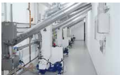
Machine-assigned sprue mills sited on the floor underneath the injection moulding area
