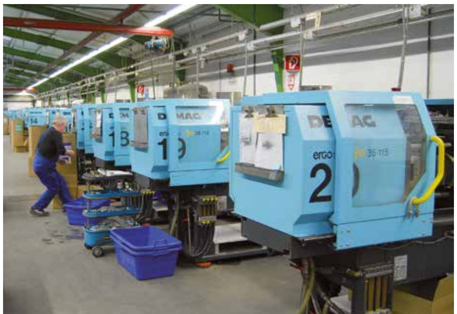
At the moment, 145 injection moulding machines are in use for 1- and 2-component technology in Bad Oeynhausen, of which only two are not from Sumitomo (SHI) Demag.
