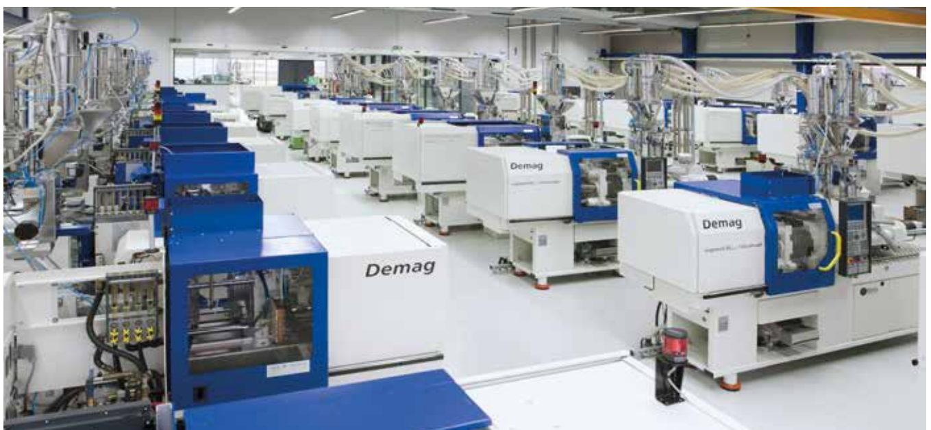
Hygiene area with well accessible injection moulding machines, arranged in rows and slightly raised for easy floor cleaning
