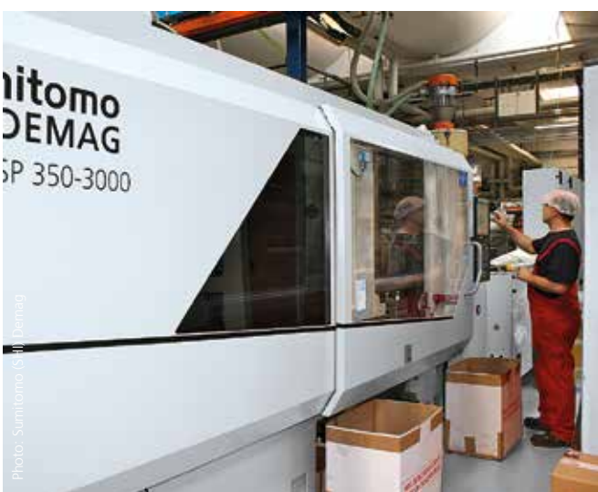
The EI-Exis SP 350-30000 manufactures snap-on lids in a 24-cavity mould.
