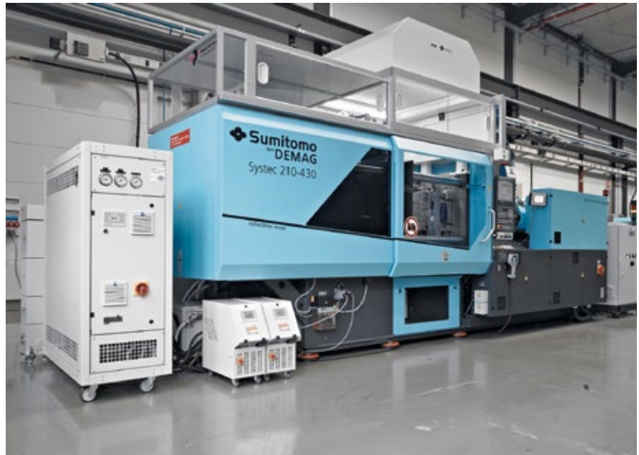
The manufacturing cell was designed around a 2,100kN Systec machine. Energy-efficient production is ensured by the dynamic power adjustment of the hydraulic drive via activeDrive, a combination of a frequency-controlled electric motor and a highly dynamic variable capacity pump.
