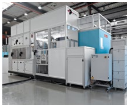
Numerous modules for robot, foil handling, clean room, automation enclosure, conveyor as well as foil cleaning and UV hardening are working together efficiently within one cell.
