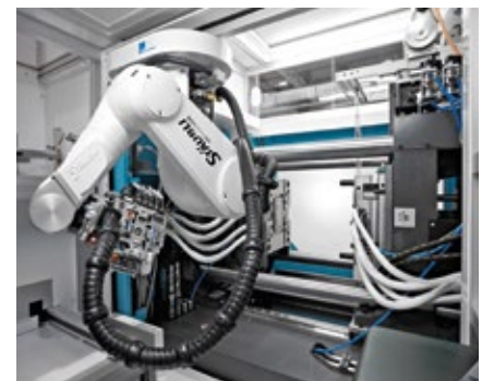
A single suspended robot with a multi-sided gripper system performs all the handling tasks involving the component and the functional label.
