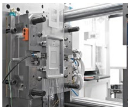
The endless carrier foil with decorative coating which passes downwards through the mould, is aligned accurately within the mould.
