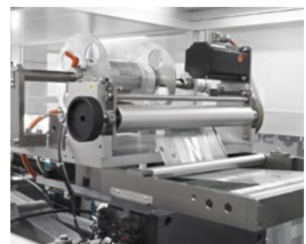
The foil feed unit from Kurz which is located above the mould, ensures the accurate positioning of the decorative foil.
