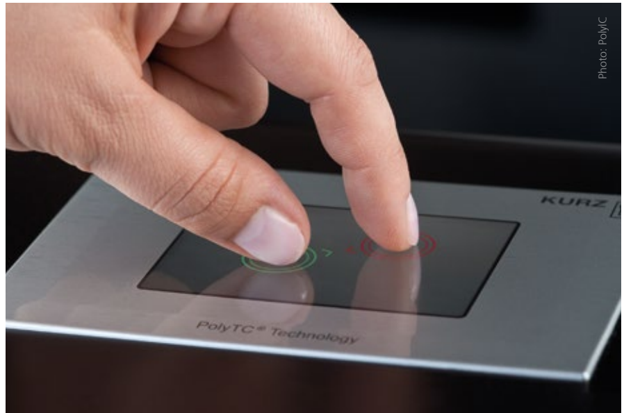
Touch functionality via IML, decoration via IMD. The two processes have been combined to manufacture this multi-touch display in a single shot.
