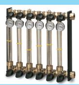
The high temperature flow regulator unit is available with an option of 2 to 8 channels with a maximum temperature of 100  $^{\circ}$ C respectively high pressure and has a flow rate of 0 – 30 l/min for each channel.
